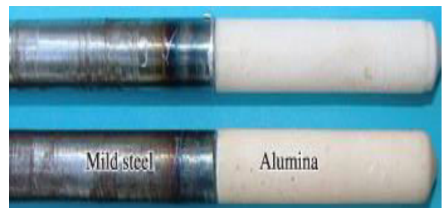
Figure 3.2: Alumina and steel weld joints
